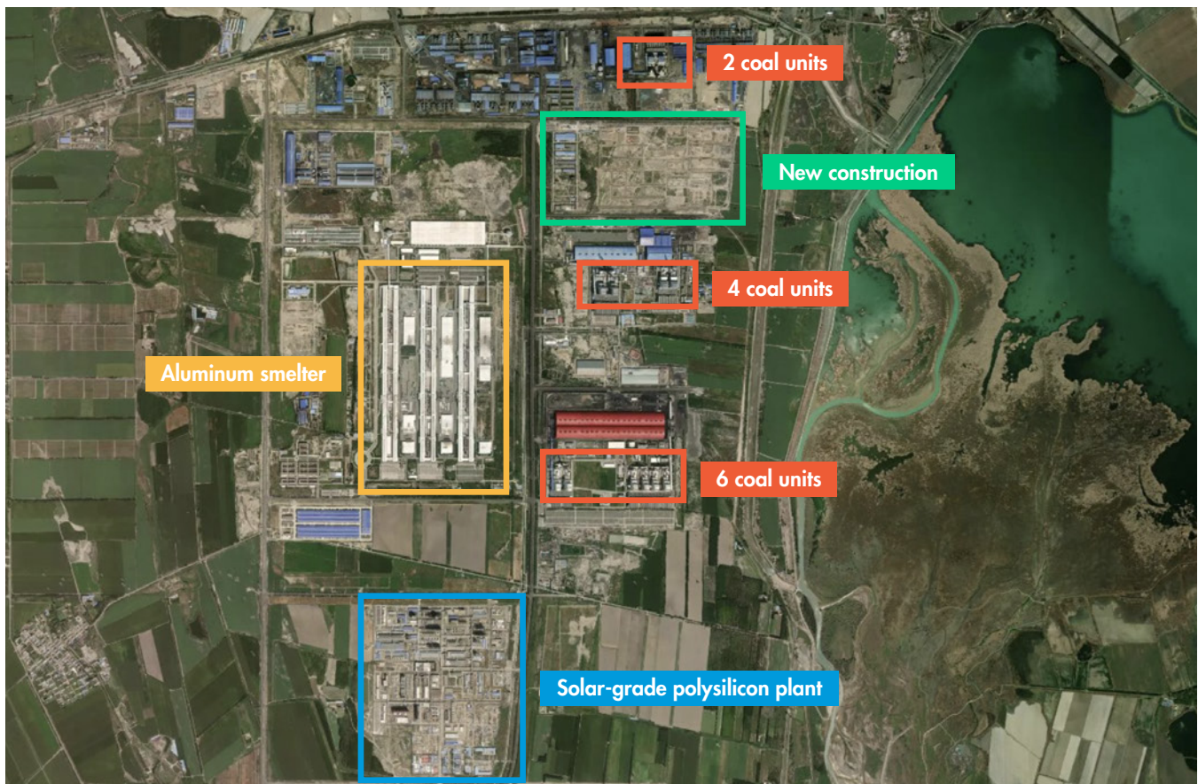
Figure 7: Satellite imagery of the solar-grade polysilicon plant operated by Daqo New Energy Corporation (44.41°N, 86.08°E) north of Shihezi, co-located with aluminum production. Visible coal power infrastructure is highlighted in red. A new expansion site for silicone production is under construction for the north, still partially incomplete as of 2022. Note that Xinjiang Western Hoshine Silicon Industry Co., Ltd., operates a metallurgical-grade silicon factory directly adjacent and to the north of this construction site, powered by the two coal units pictured. Imagery is captured from the Mapbox satellite product ( https://josm.openstreetmap.de/mapsview?entry=Mapbox%20Satellite ), and dates from after 2018.
