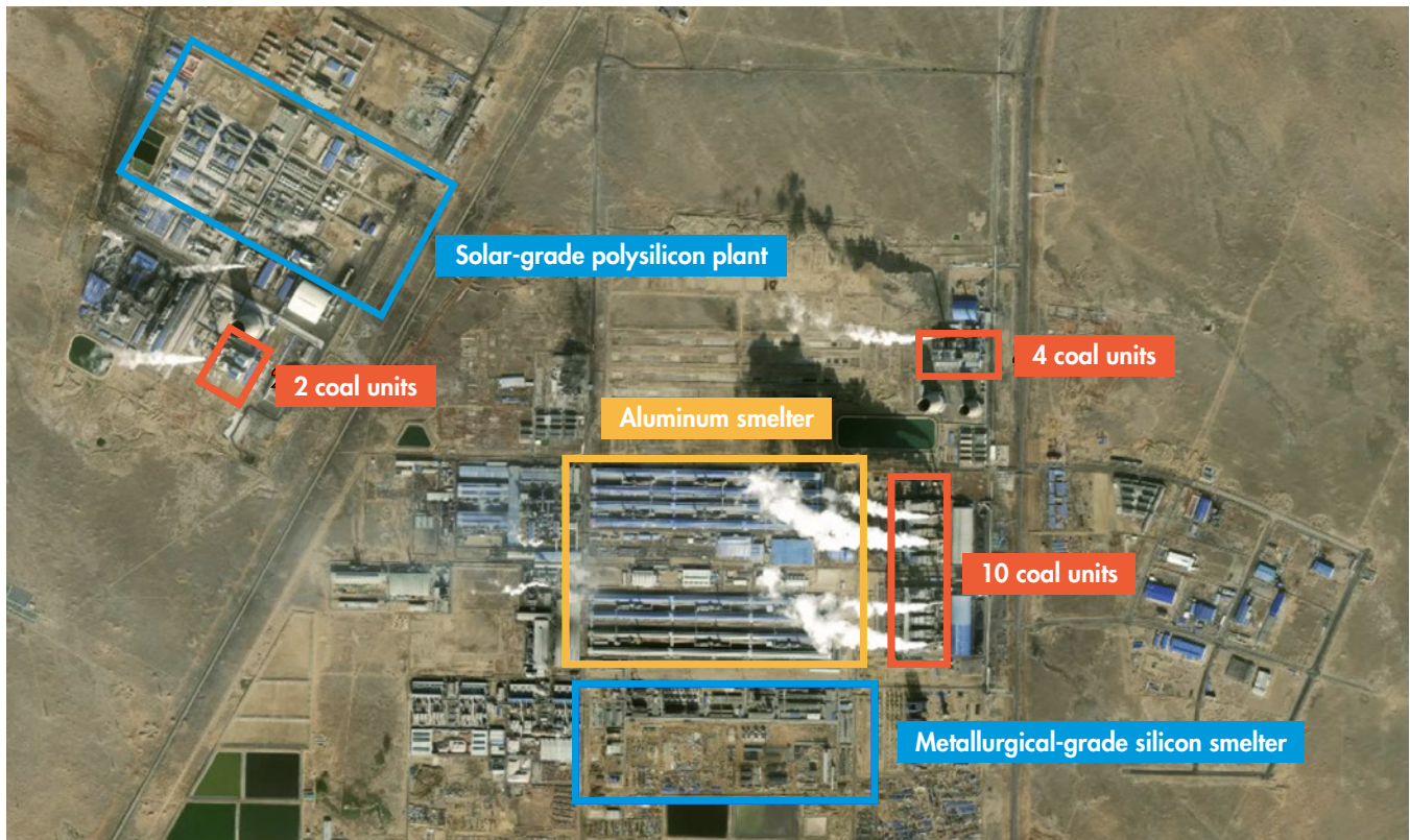
Figure 6: Satellite imagery of the solar-grade polysilicon plant operated by East Hope Group (44.68°N, 89.10°E) in the Zhundong Economic and Technological Development Zone and co-located with aluminum production. Visible coal power infrastructure is highlighted in red. Imagery is captured from the Mapbox satellite product ( https://josm.open-streetmap.de/mapsview?entry=Mapbox%20Satellite ), and dates from after 2018.
